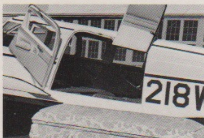
New optional utility door provides a loading entrance almost 5 feet wide at a convenient loading level.
