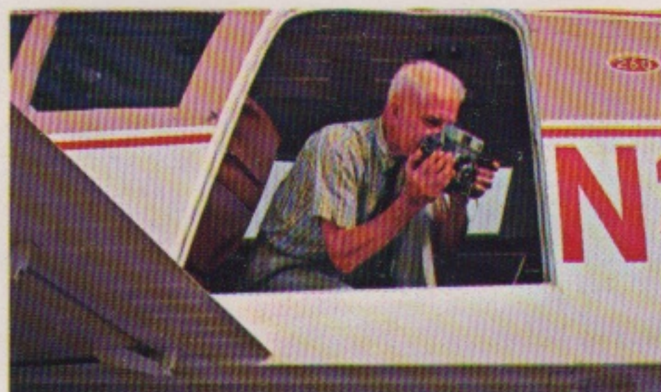
FAA-approved for flight with rear passenger door removed. Great for dropping supplies, parachutists, aerial photography.
