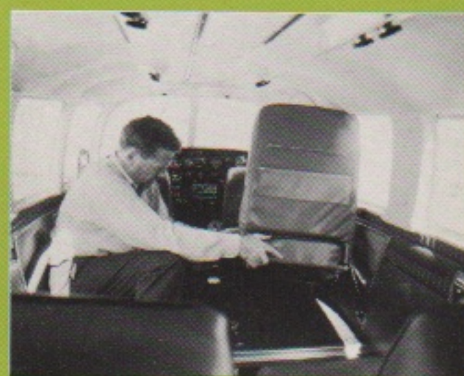
QC! Seats remove in seconds, without any tools whatsoever.
